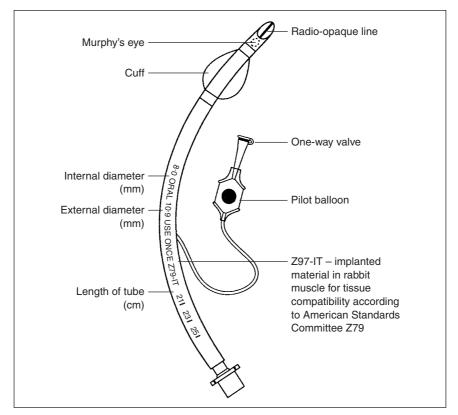
Figure 2.2 Typical endotracheal tube.
